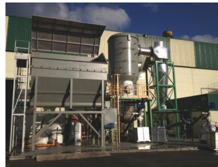
MBM Gasifier Plant 10 MWth steam. Salamanca, España
